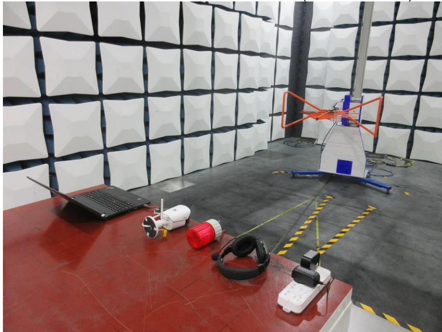
RADIATED RF MEASUREMENT SETUP (30MHz ~ 1 GHz)
