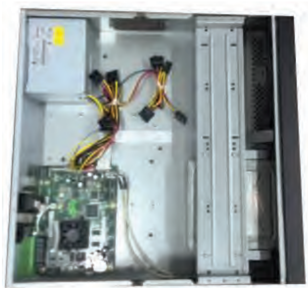
Figure 3-40 Put bracket back
