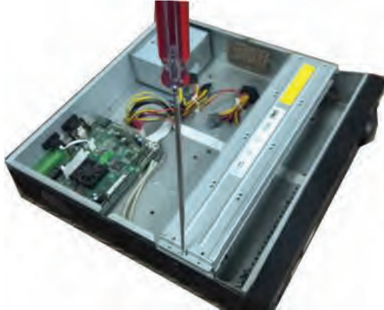
Figure 3-32 Open the top cover
