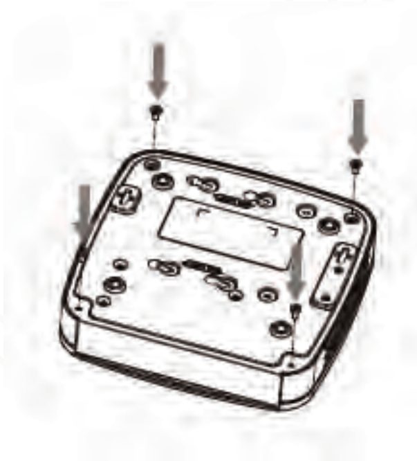
Figure 3-6 Put back the cover
