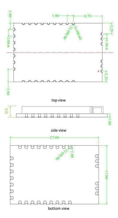
Figure 6 Module dimension (top , side and bottom view)
