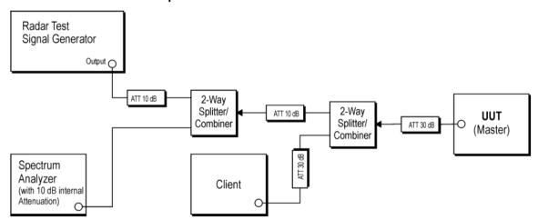
Remark: During the test, a lower radar signal level -55.09dBm was used.
