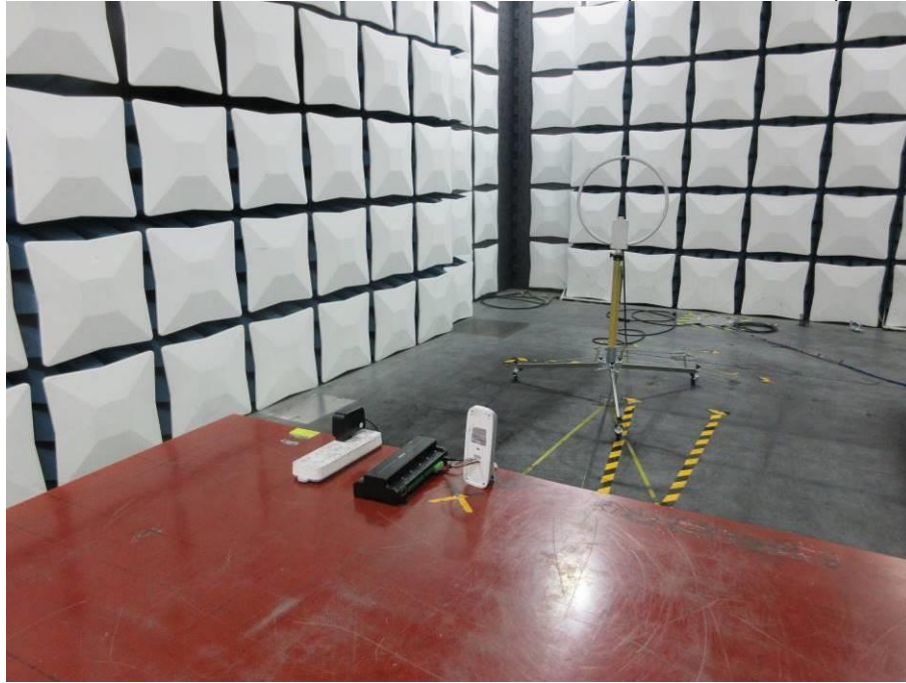
RADIATED RF MEASUREMENT SETUP (9kHz ~ 30 MHz)
