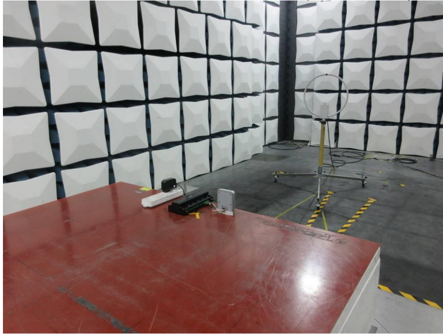
RADIATED RF MEASUREMENT SETUP (9kHz ~ 30 MHz)
