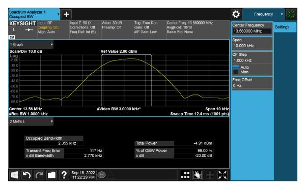
Note: Because the measured signal is CW or CW-like adjusting the RBW per C63.10 would not be practical since measured bandwidth will always follow the RBW and the result will be approximately twice the RBW. And the signal was narrowband, therefore it was impossible to set RBW within 1% ~ 5%.
