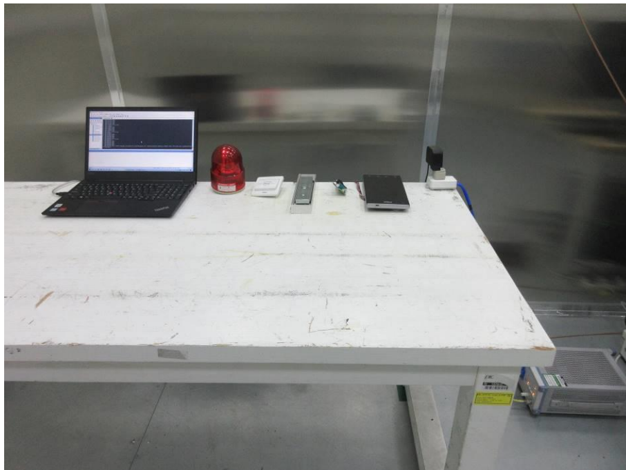
POWERLINE CONDUCTED EMISSIONS MEASUREMENT SETUP
