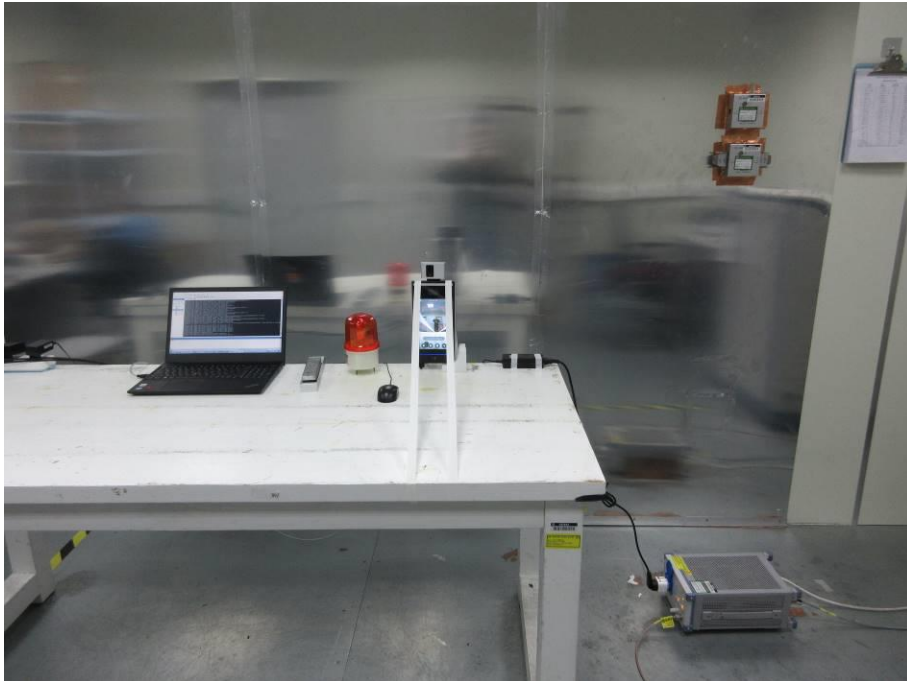
POWERLINE CONDUCTED EMISSIONS MEASUREMENT SETUP
