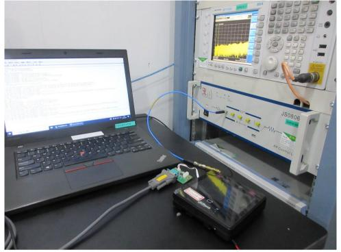
Radiated Spurious Emissions (9kHz-30MHz)
