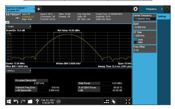
Note: 1. Because the measured signal is CW or CW-like adjusting the RBW per C63.10 would not be practical since measured bandwidth will always follow the RBW and the result will be approximately twice the RBW. And the signal was narrowband, therefore it was impossible to set RBW within 1% ~ 5%.
