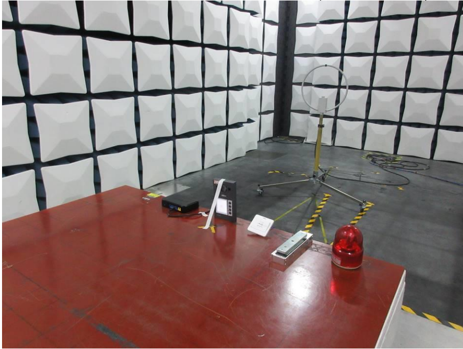
RADIATED RF MEASUREMENT SETUP (9kHz ~ 30 MHz)
