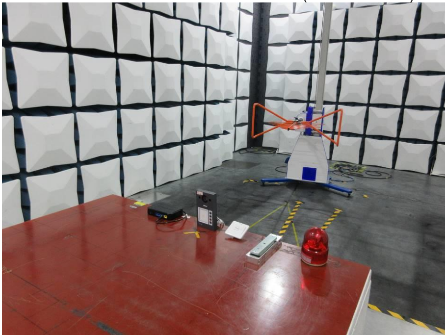
RADIATED RF MEASUREMENT SETUP (30MHz ~ 1 GHz)
