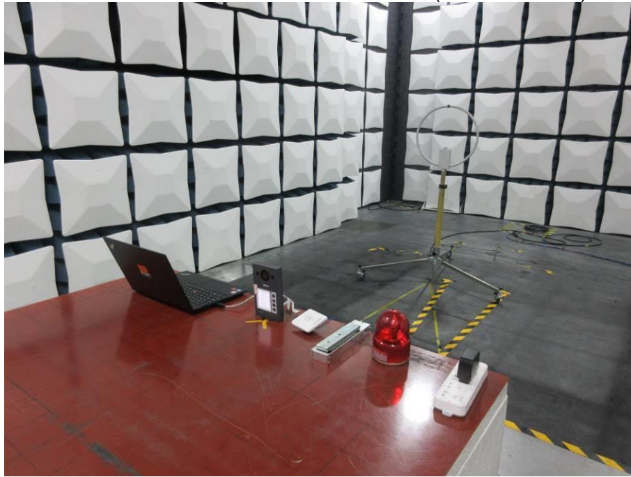
RADIATED RF MEASUREMENT SETUP (9kHz ~ 30 MHz)
