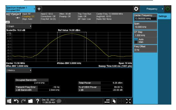
Remark: Because the measured signal is CW or CW-like adjusting the RBW per C63.10 would not be practical since measured bandwidth will always follow the RBW and the result will be approximately twice the RBW. And the signal was narrowband, therefore it was impossible to set RBW within  $1\% \sim 5\%$ .
