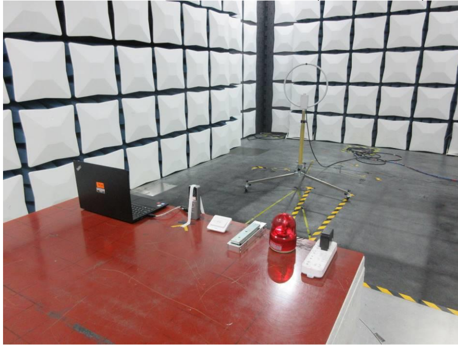
RADIATED RF MEASUREMENT SETUP (9kHz ~ 30 MHz)
