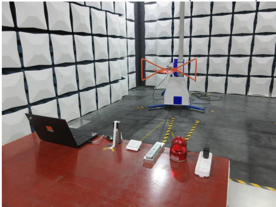
RADIATED RF MEASUREMENT SETUP (30MHz ~ 1 GHz)
