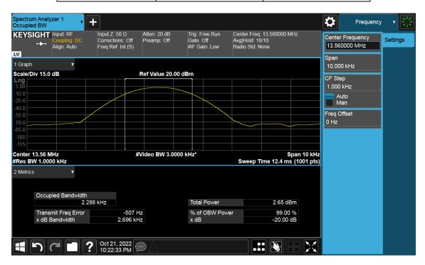
Note: Because the measured signal is CW or CW-like adjusting the RBW per C63.10 would not be practical since measured bandwidth will always follow the RBW and the result will be approximately twice the RBW. And the signal was narrowband, therefore it was impossible to set RBW within 1% ~ 5%.
