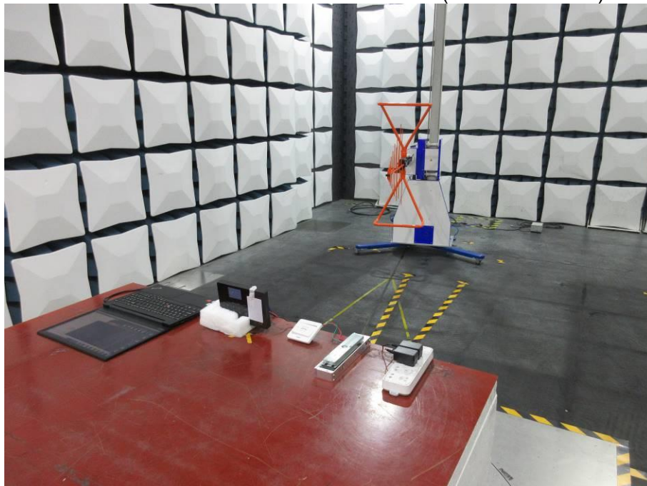
RADIATED RF MEASUREMENT SETUP (30MHz ~ 1 GHz)
