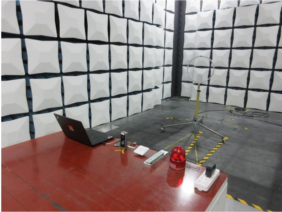
RADIATED RF MEASUREMENT SETUP (9kHz ~ 30 MHz)
