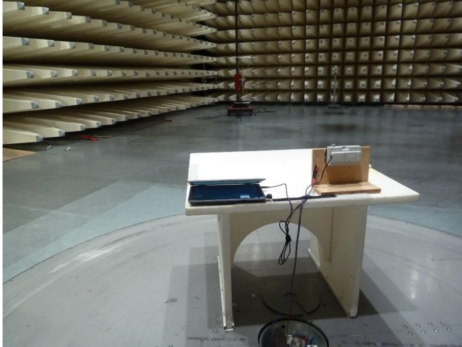
Photo 1 (RSE setup 30 MHz to 1 GHz – EUT with control PC):
