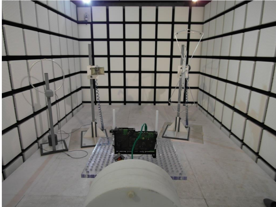
Photo 3 - Spurious Emissions 30MHz to 1 GHz EUT Set-up with internal antenna:
