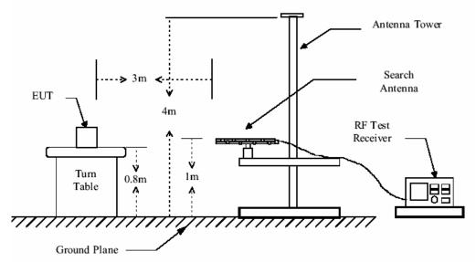
Radiated Emission Test Set-up Frequency Over 1GHz
