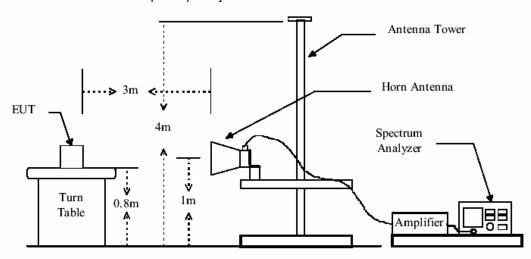
Low nosie amplifier was used below 1GHz, High pass Filter was used above 1GHz.
