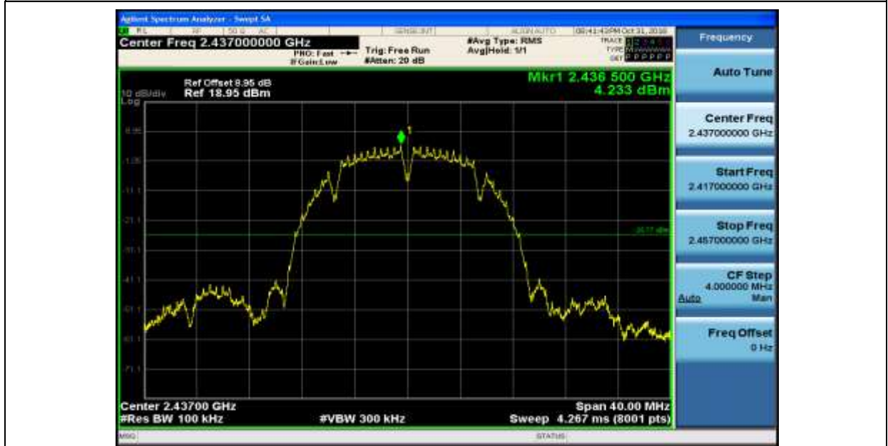
RF Conducted Spurious Emissions_11B_2437
