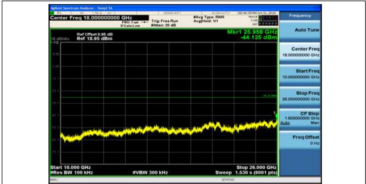
RF Conducted Spurious Emissions_11G_2412
