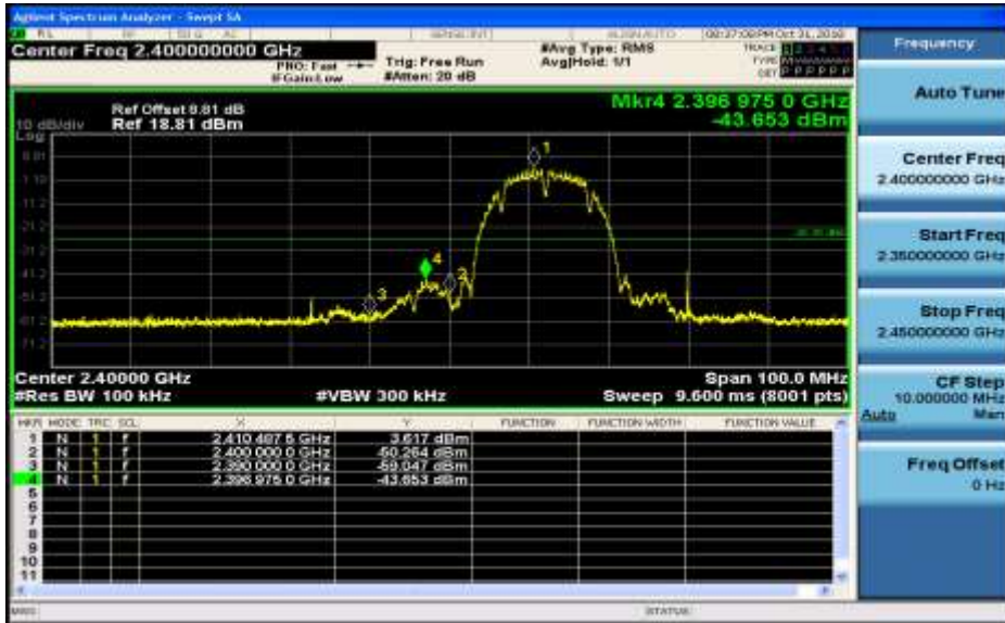
Band-edge for RF Conducted Emissions_11B_2462_Ant1
