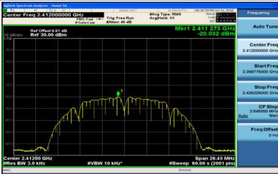
Maximum(average) power spectral density_11B_2437_Ant1
