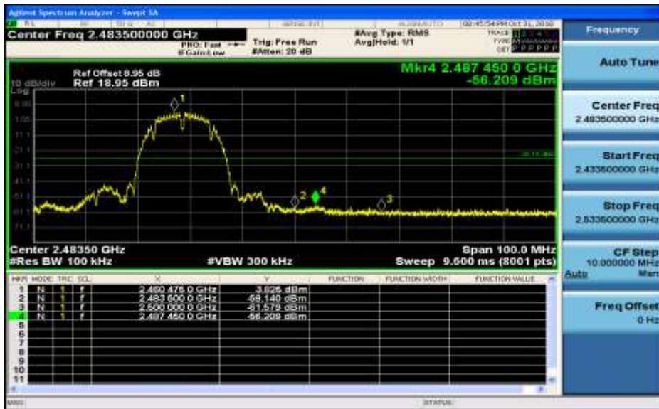
Band-edge for RF Conducted Emissions_11G_2412_Ant1
