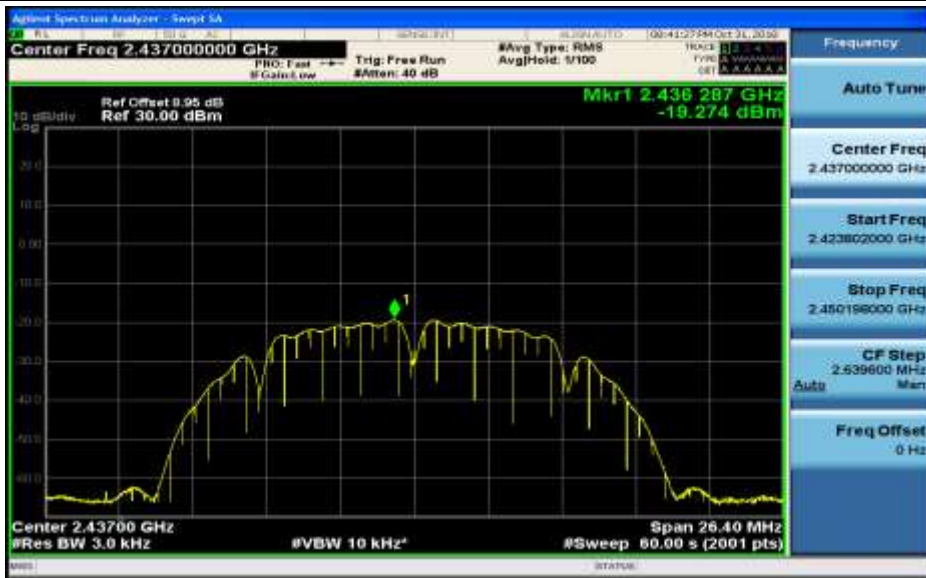
Maximum(average) power spectral density_11B_2462_Ant1
