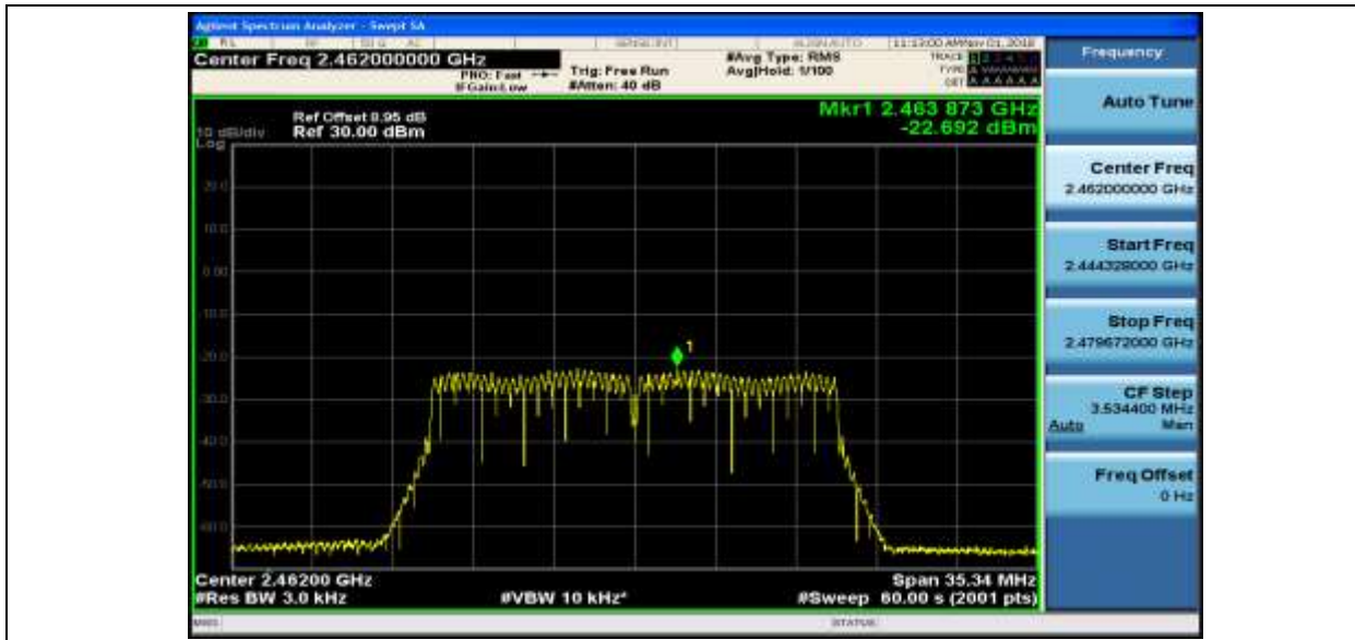
Maximum(average) power spectral density_11N40SISO_2422_Ant1
