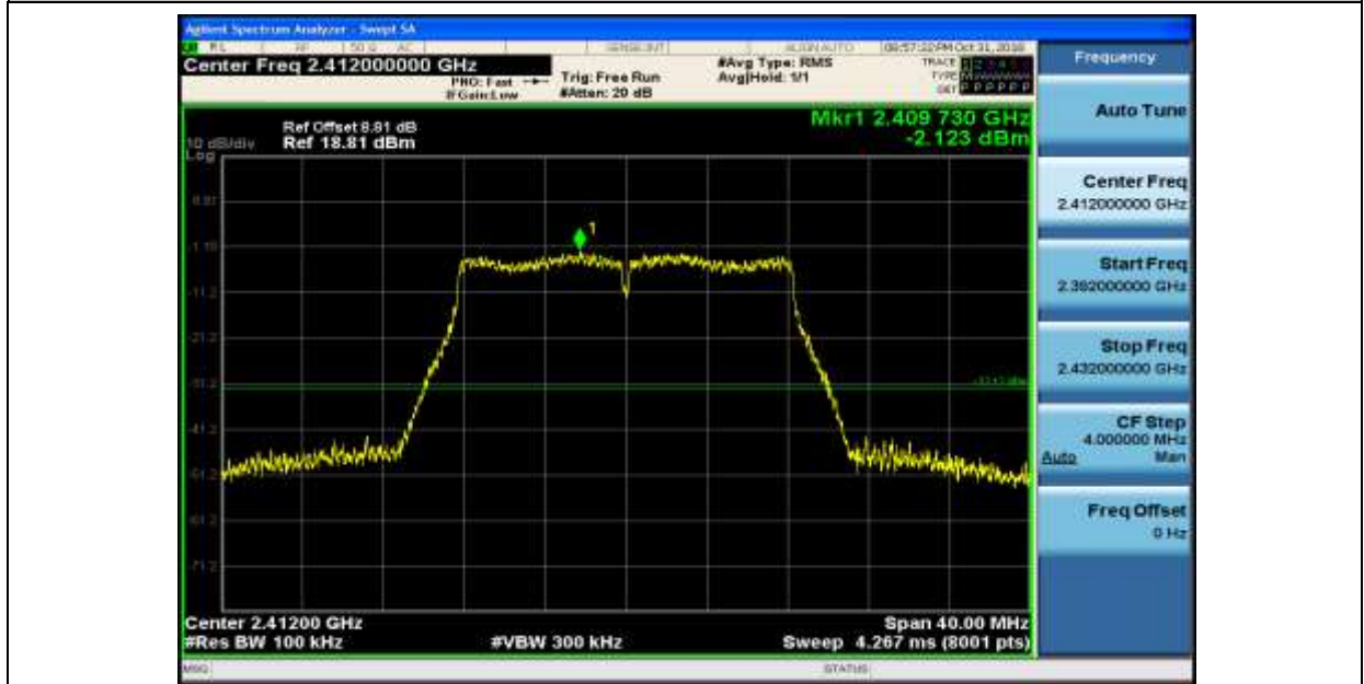
RF Conducted Spurious Emissions_11G_2412
