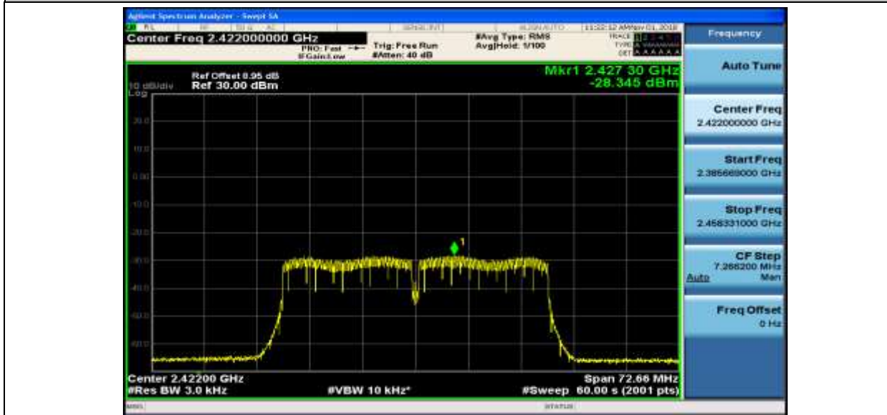
Maximum(average) power spectral density_11N40SISO_2437_Ant1
