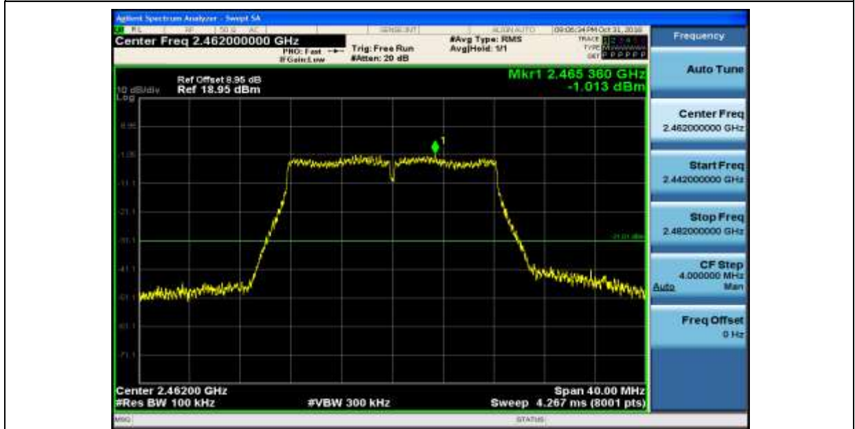
RF Conducted Spurious Emissions_11G_2462
