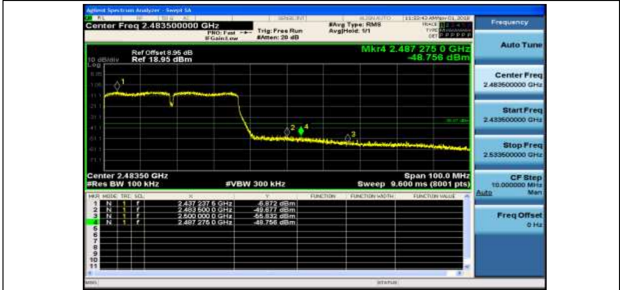
Band-edge for RF Conducted Emissions_11N40SISO_2452_Ant1
