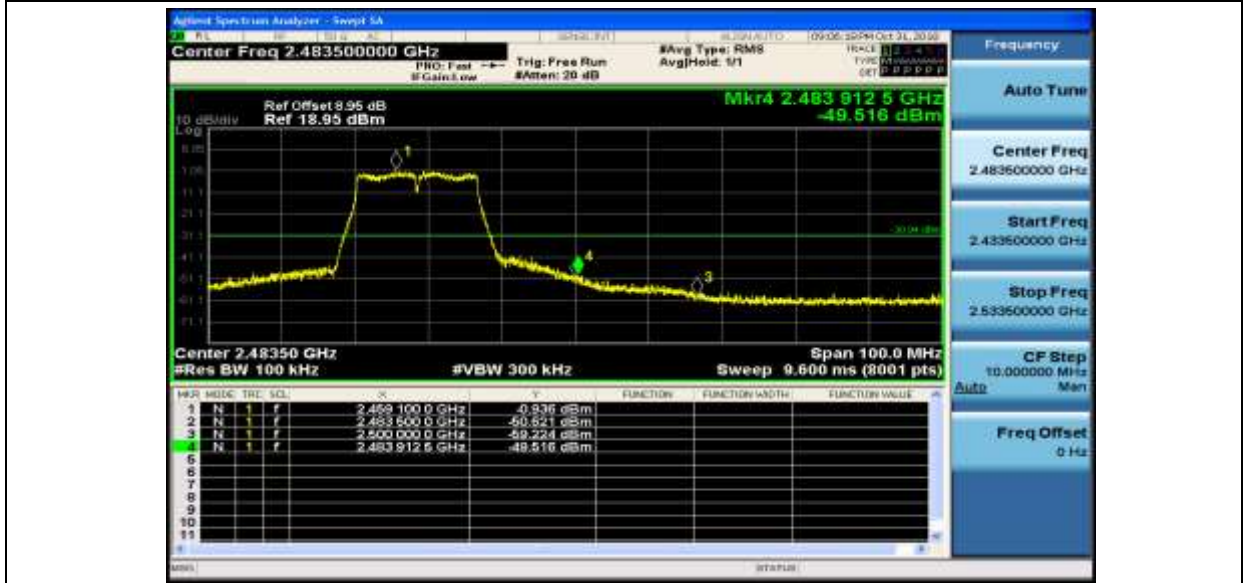
Band-edge for RF Conducted Emissions_11N20SISO_2412_Ant1
