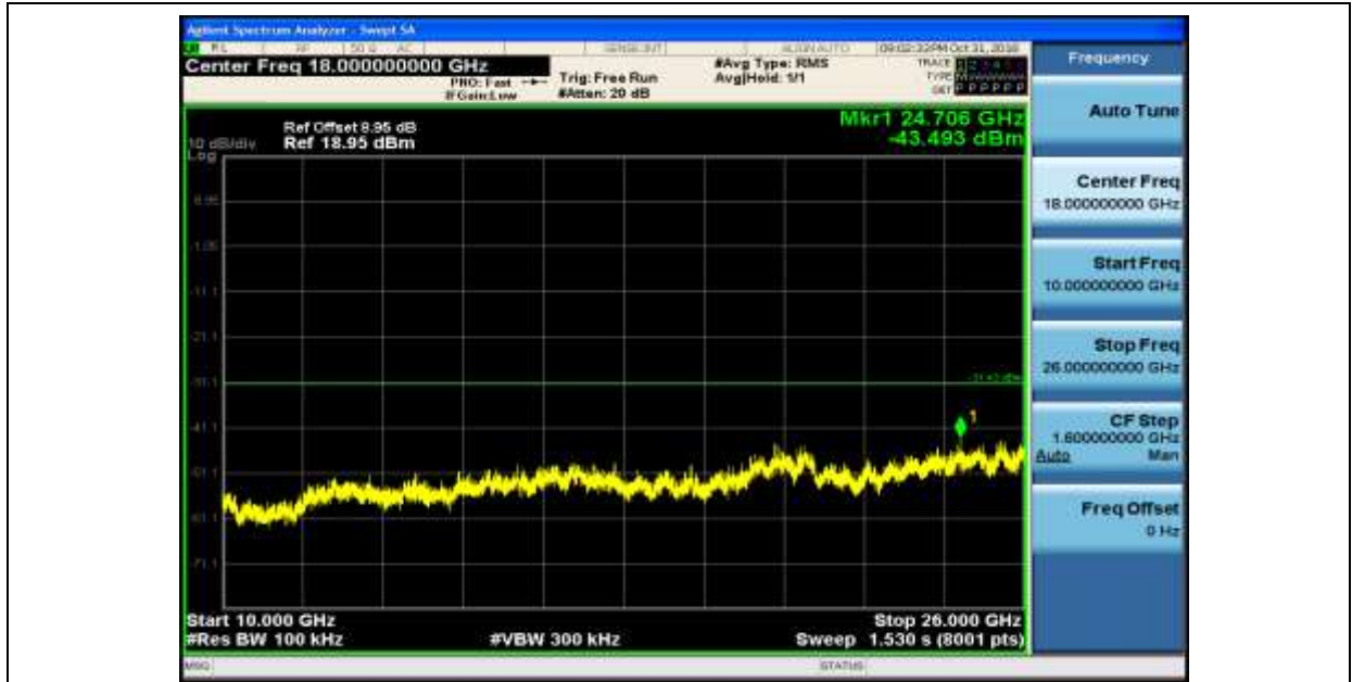
RF Conducted Spurious Emissions_11G_2462
