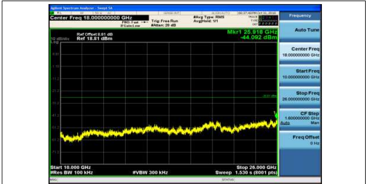
RF Conducted Spurious Emissions_11B_2437
