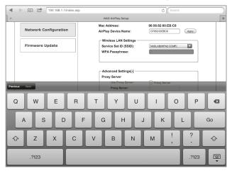
6 A Warning notice will pop-up. Select **OK** to save the new settings. The flashing signal bar indicator **ull** turns to solid bar. Your iOS device (iPad) is now interfaced with the D 7050.
