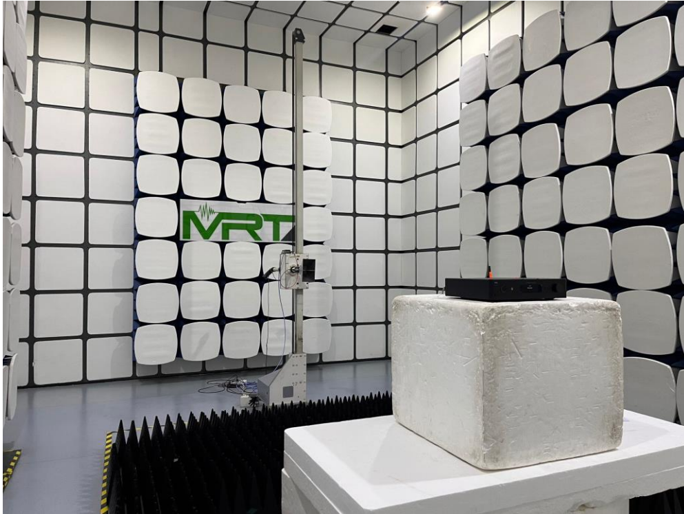
Description: Radiated Spurious Emission Test Setup for Above 18GHz
