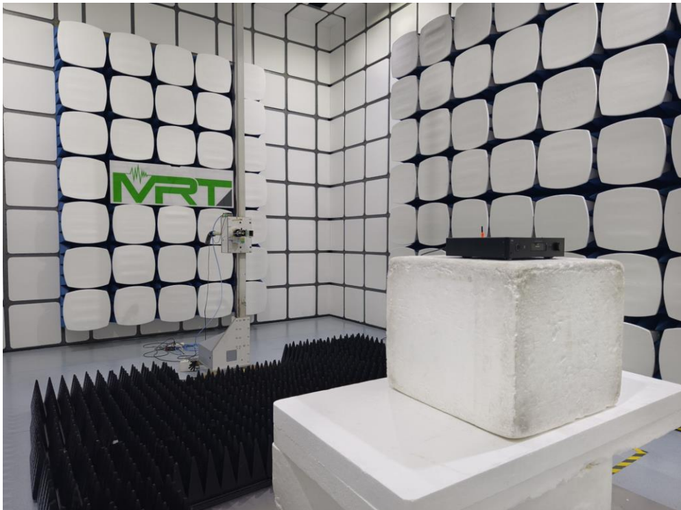
Description: Radiated Spurious Emission Test Setup for Above 18GHz
