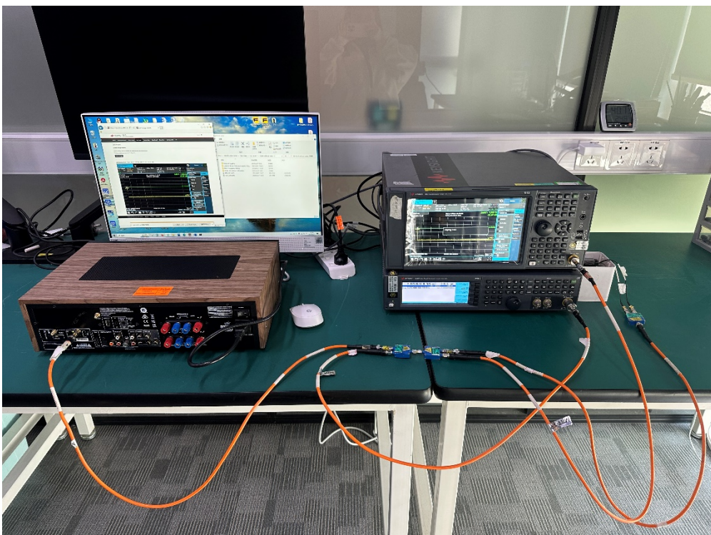
Description: Dynamic Frequency Selection Measurement Test Setup
