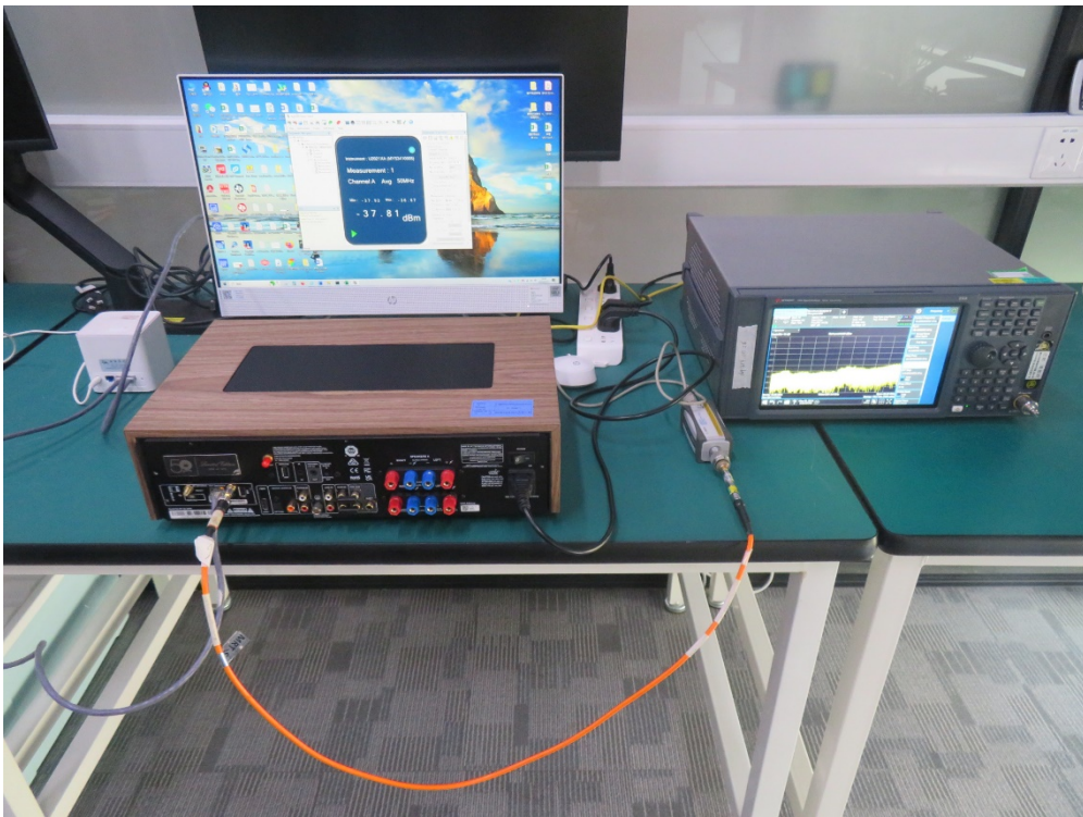
Description: Dynamic Frequency Selection Measurement Test Setup
