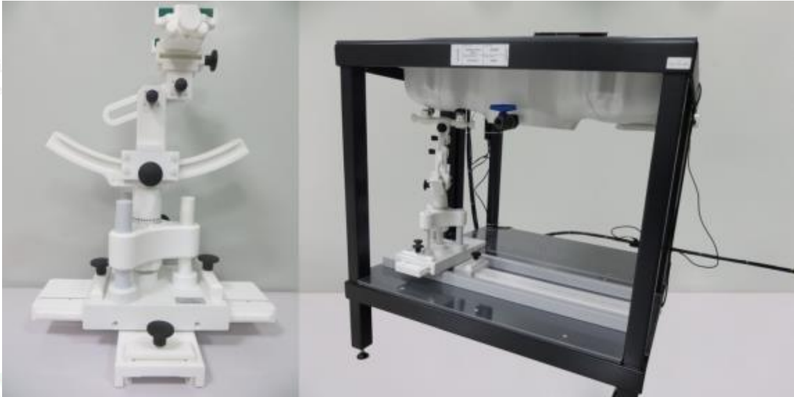
Device holder supplied by SATIMO
