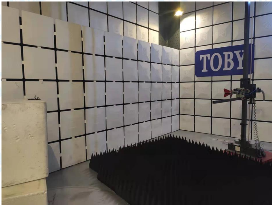
Photo of Setup for Conducted Emission
