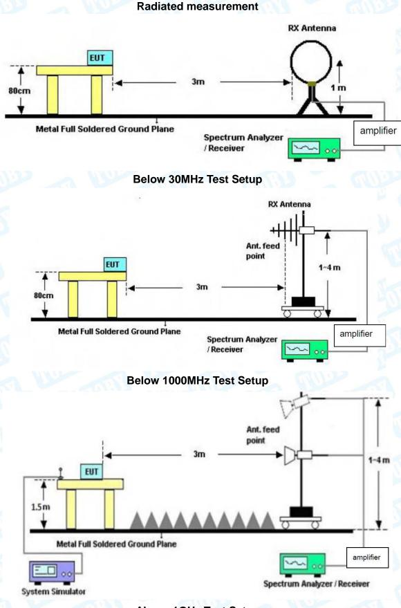
Above 1GHz Test Setup
