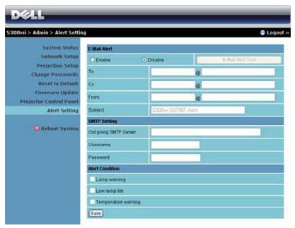
E-mail Alert: With standard SMPT server using default 25 port and not support encryption and authentication (SSL or TLS).
