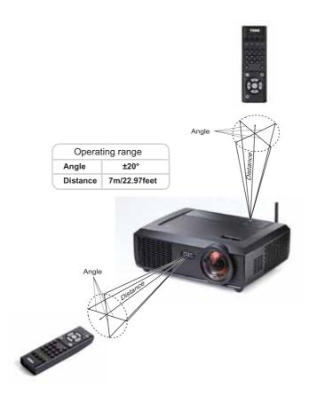
**NOTE:** Actual operating range may slightly differ from the diagram. Weak batteries will also prevent the remote control from properly operating the projector.
