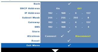
**DHCP ADDRESS**—If a DHCP server exists in the network to which the projector is connected, the IP address will automatically be acquired when you select DHCP On. If DHCP is Off, manually set the IP Address, Subnet Mask, and Gateway. Use to select the number of IP Address, Subnet Mask, and Gateway. Key in Enter to confirm each number and then use  $\boxtimes$  to set the next item.
