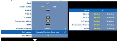
**VGA-A**—Use **<** and **>** to enable or disable VGA-A input.
