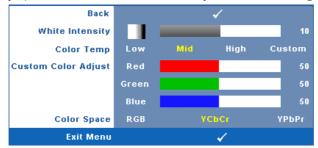
**COLOR TEMP**—Allows you to adjust the color temperature. The screen appears cooler at higher color temperatures and warmer at lower color temperatures. When you adjust the values in the **Color Adjust** menu, the Custom mode is activated. The values are saved in the Custom mode.
