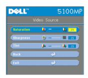
**SATURATION**—Adjust a video source from black and white to fully saturated color. Press  $\bigcirc$  to decrease the amount of color in the image and  $\bigcirc$  to increase the amount of color in the image.
