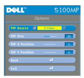
**PIP IMAGE** —Select On to enter Options to select following settings. Select Off to disable the picture-in-picture display function.
