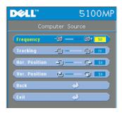
**FREQUENCY**—Change the display data clock frequency to match the frequency of your computer graphics card. If you see a vertical flickering bar, use Frequency control to minimize the bars. This is a coarse adjustment.
