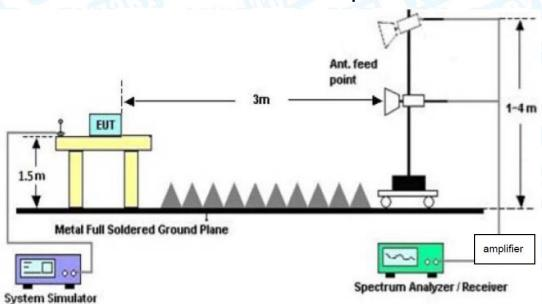
**Above 1GHz Test Setup**
