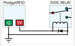
Make sure to attach a diode across the terminals of the relay if you are using output 0 on the RFID board to drive it.
