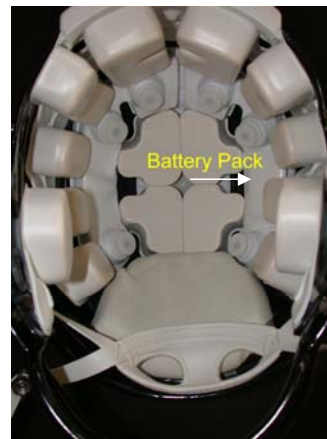
Figure 7: Battery Pack Installed
