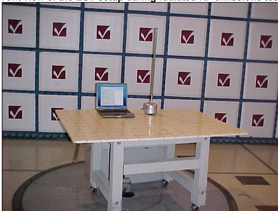
Front view of the EUT setup during radiated RF emissions tests
