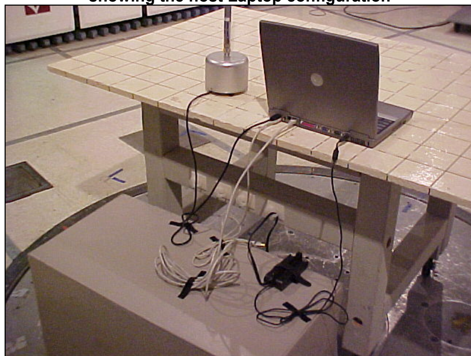
Rear view of the EUT setup during radiated RF emissions tests, showing the host Laptop configuration
