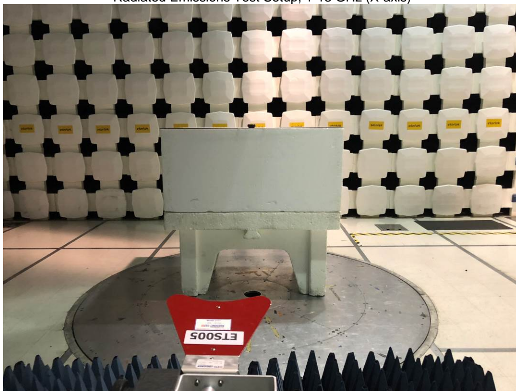
Radiated Emissions Test Setup, 1-13 GHz (X-axis)
