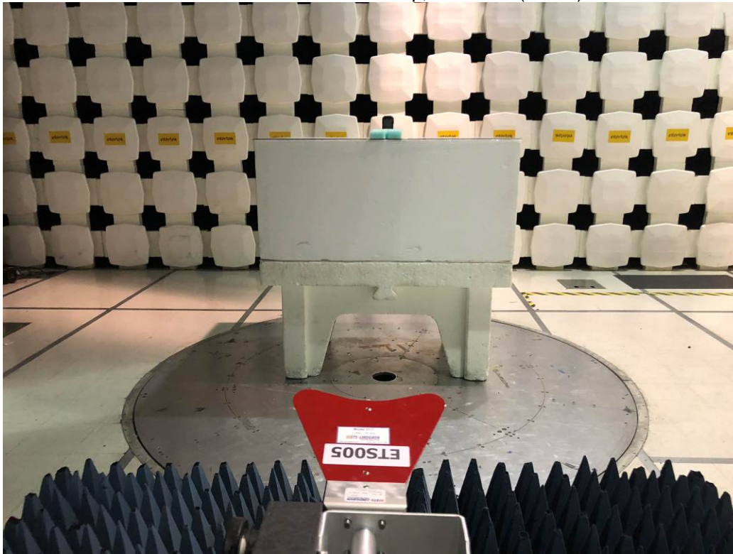
Radiated Emissions Test Setup, 1-13 GHz (Z-axis)
