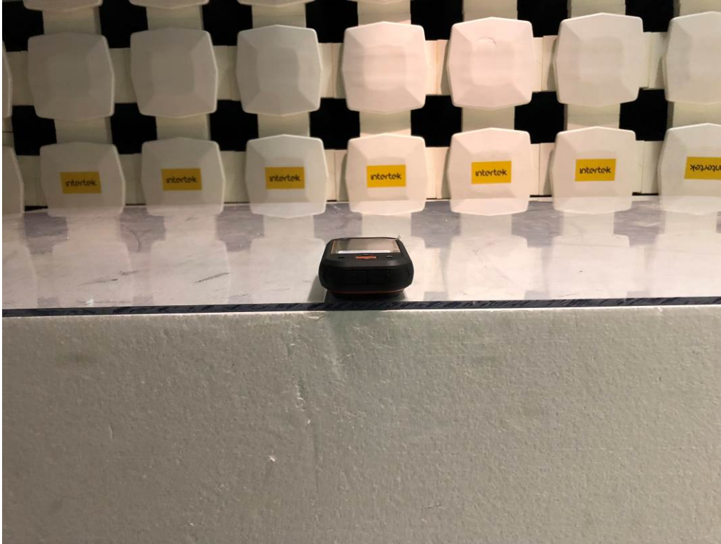
Radiated Emissions Test Setup, 30-1000 MHz (Y-axis)
