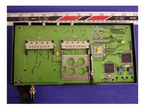
Main Board - Component View with Transceiver
