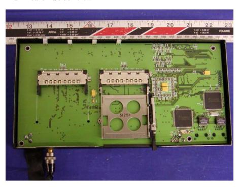
Main Board – Component View without Transceiver
