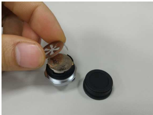
Install battery into sensor
