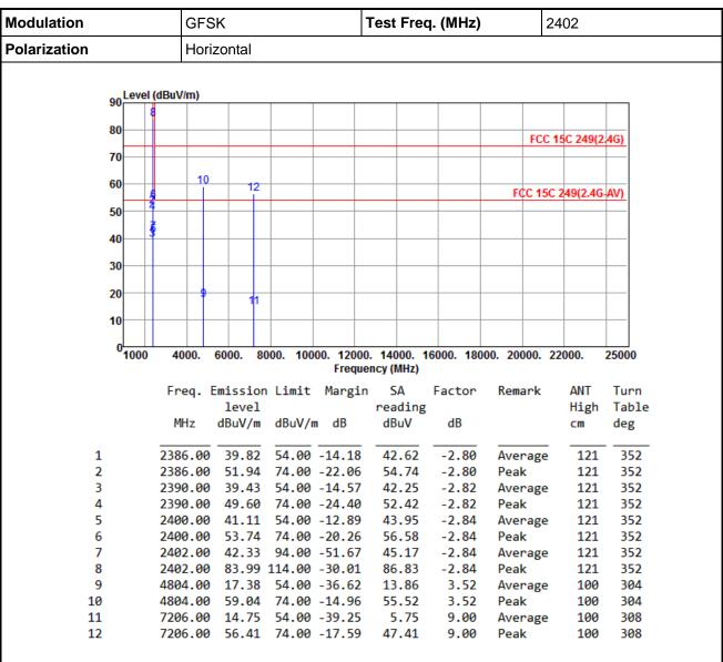
Note 1: Emission Level (dBuV/m) = SA Reading (dBuV/m) + Factor\* (dB)
