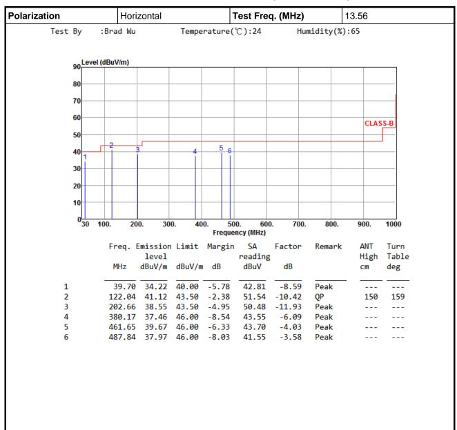
Note 1: Emission Level (dBuV/m) = SA Reading (dBuV) + Factor\* (dB)
