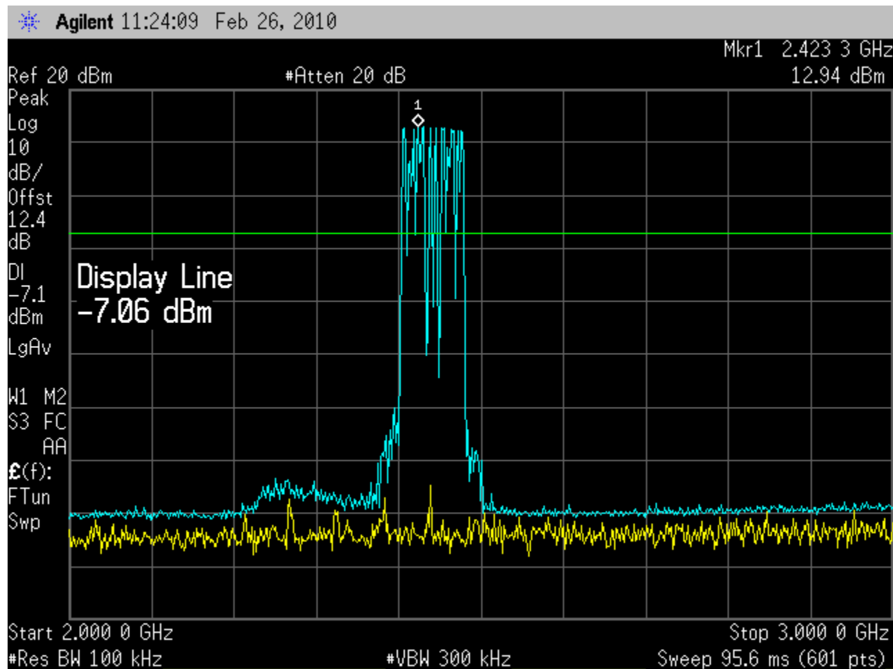
Plots from 2GHz to 3GHz , Display Line is -7.1dBm which is 20dB below the highest in band emission.
