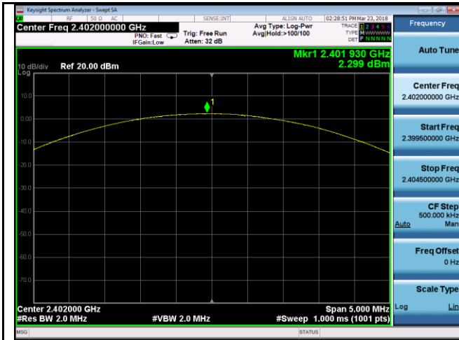
8DPSK Output power - Low CH 2402
