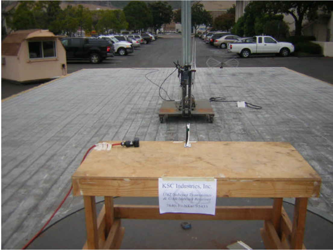
Photograph 2. Radiated Emissions Test Configuration
