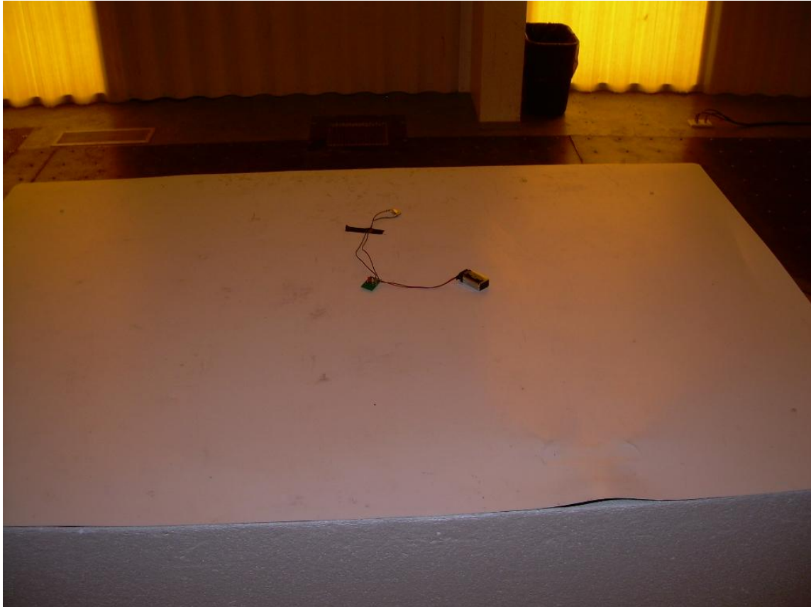
Photograph 2 – Test Configuration – Horizontal Placement of EUT
