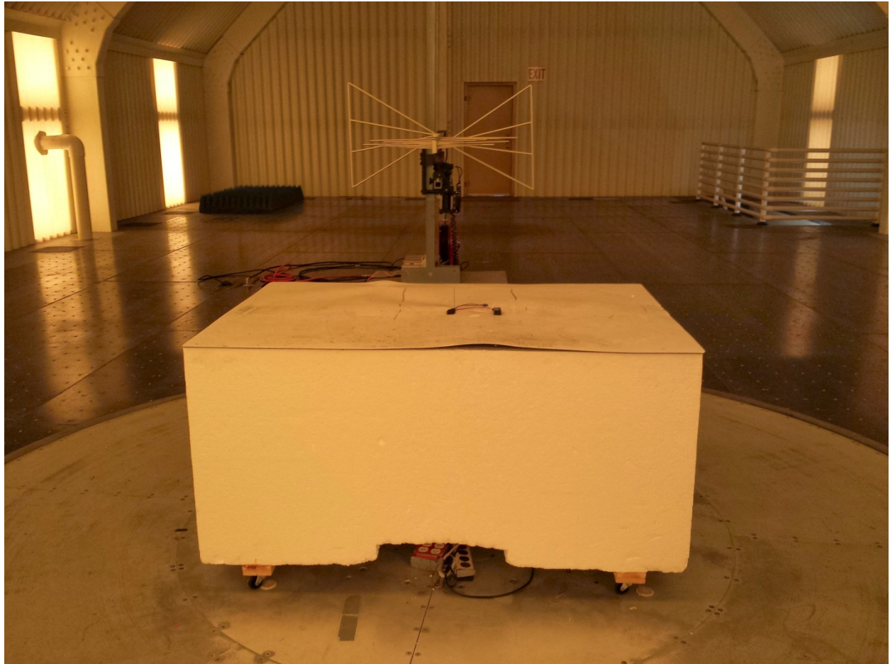
Rear View Radiated Disturbance Worst Case Configuration (Flat)
