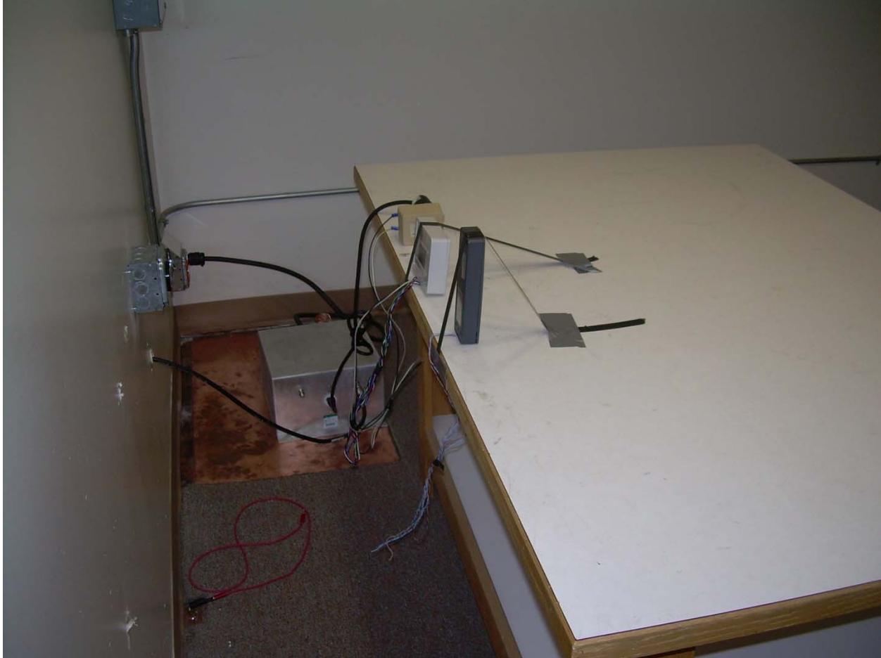
Photograph 4 – Back View Conducted Disturbance Worst Case Configuration
