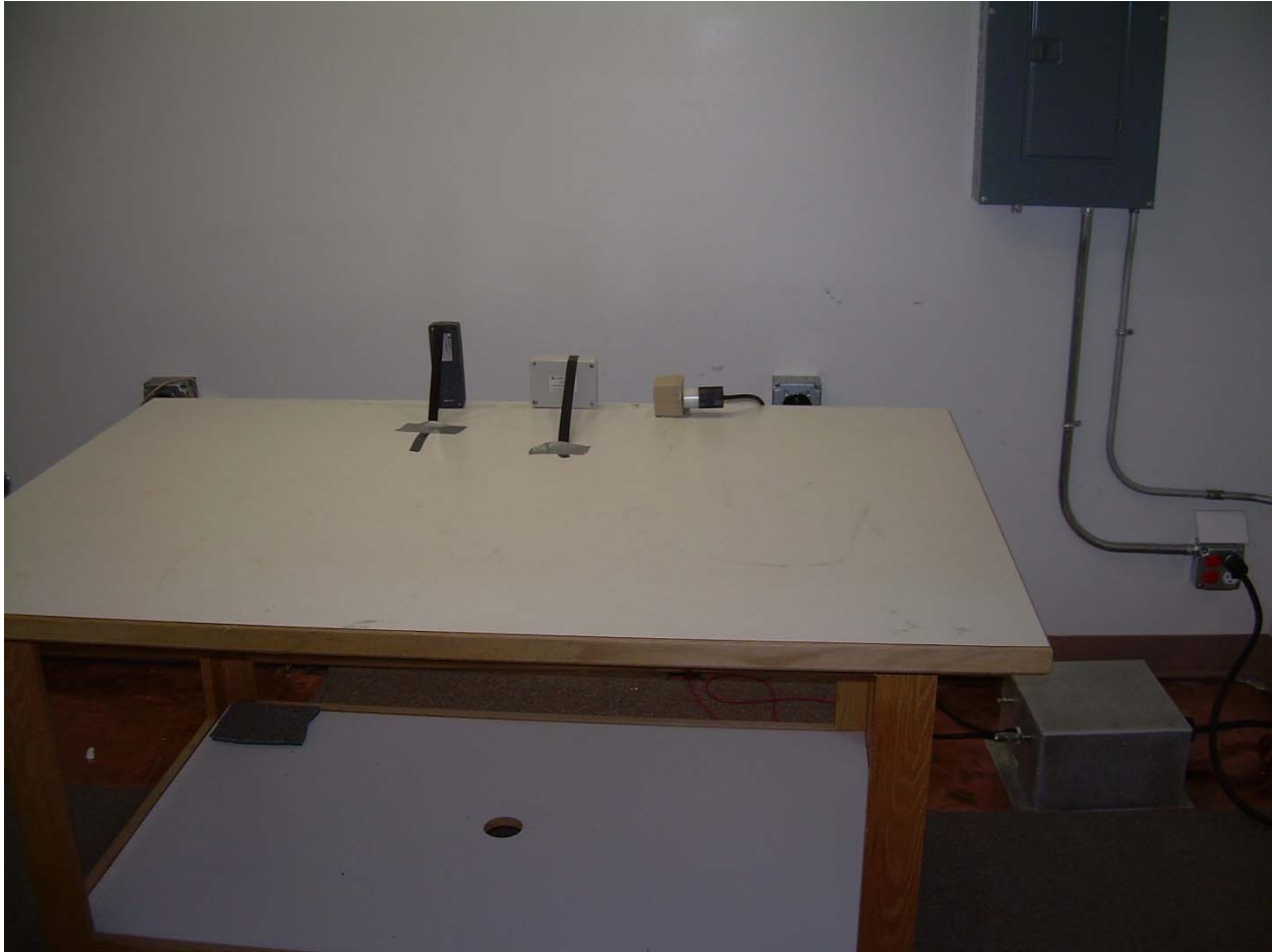
Photograph 3 – Front View Conducted Disturbance Worst Case Configuration
