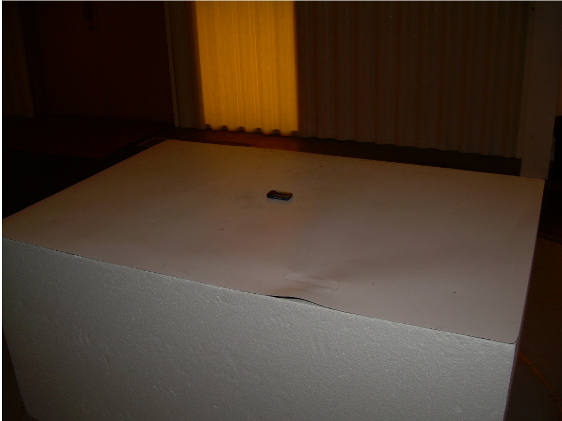
Photograph 2 – View Radiated Disturbance - Horizontal Configuration
