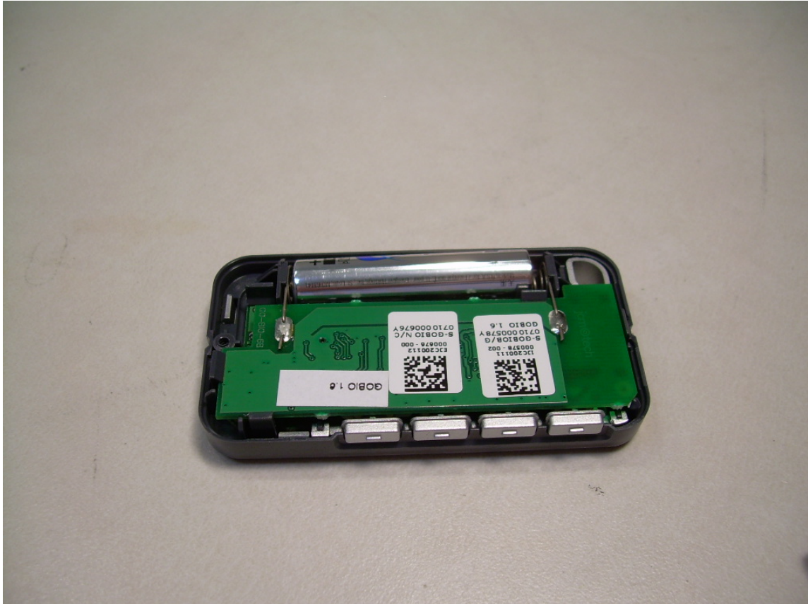
Photograph 6 – Cover Removed Showing PCB Stack in the Case
