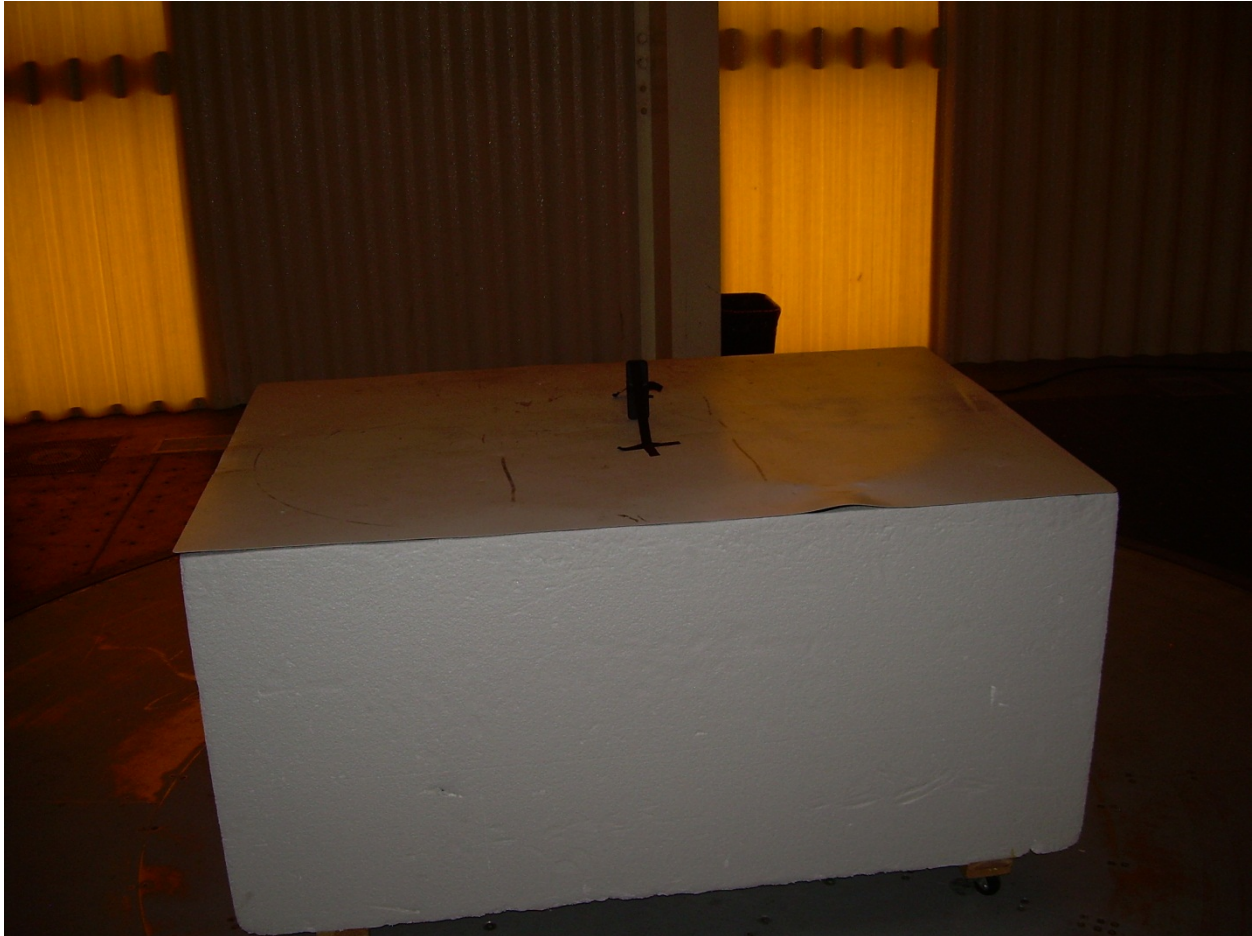
Photograph 1 – Front View Radiated Setup – Worst Case Configuration – Vertical Placement
