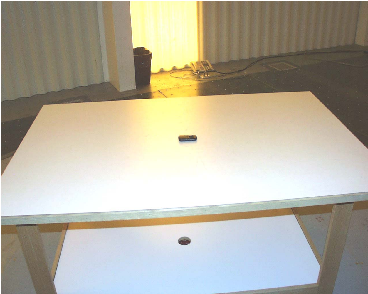
View of the Radiated Emission Test Setup (Horizontal Flat Alignment)
