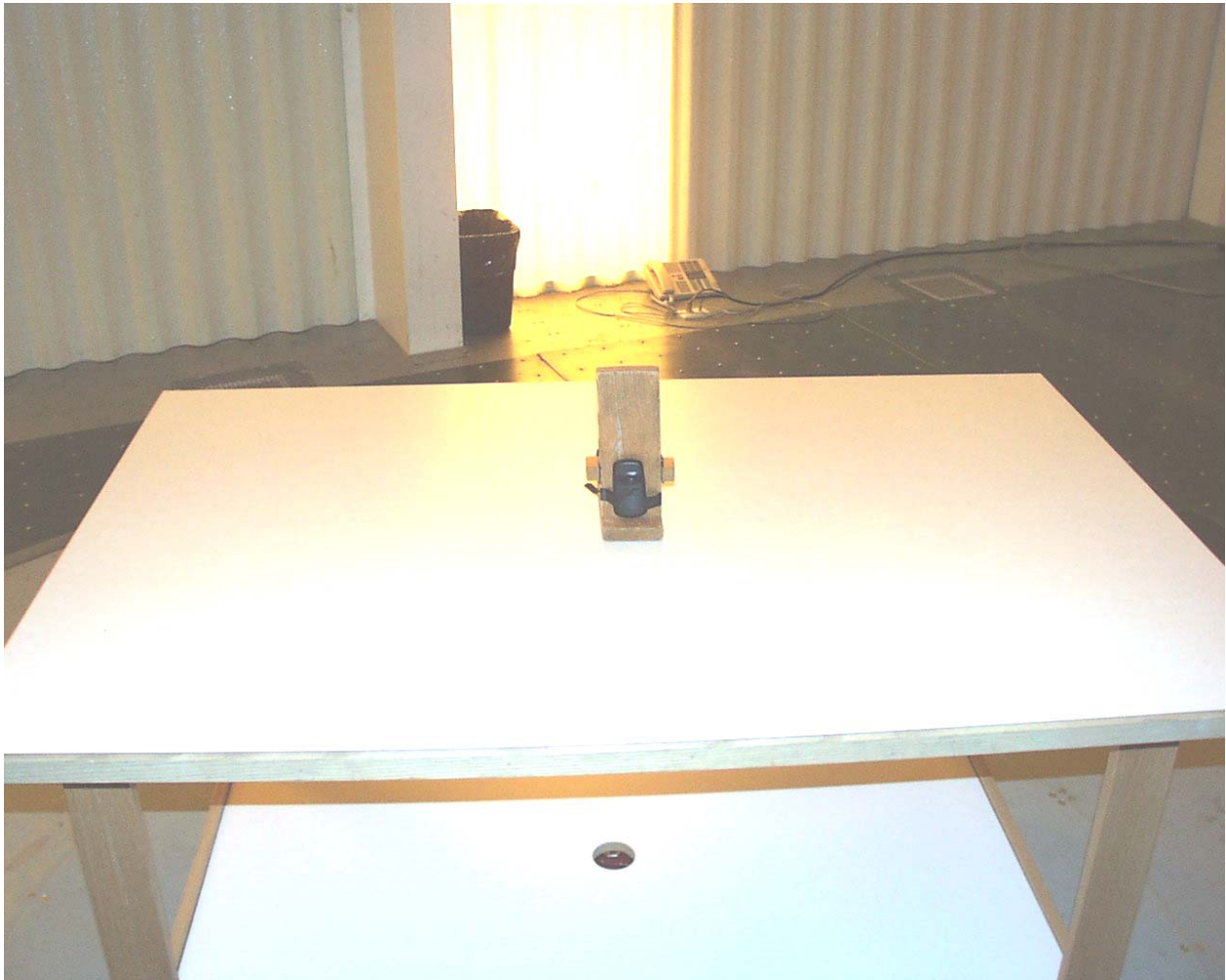
View of the Radiated Emission Test Setup (Vertical Alignment)
