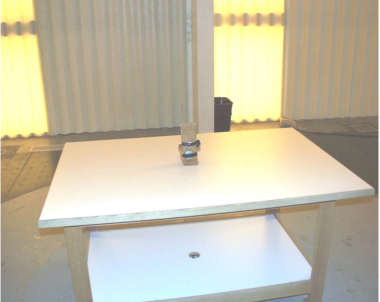
View of the Radiated Test Setup (Vertical Orientation)
