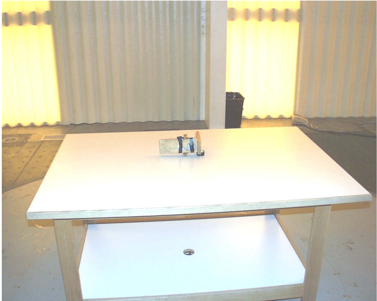
View of the Radiated Test Setup (Horizontal Orientation with Front Perpendicular to Tabletop)
